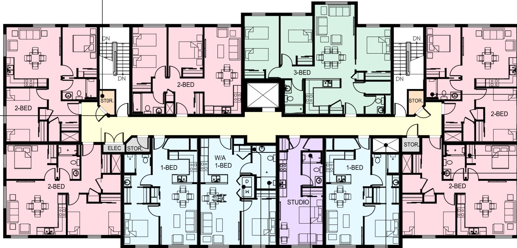
CHAMFERED WALLS CAN ASSIST IN BETTER VISIBILITY AT CORNERS TO IMPROVED SECURITY (TYP)
