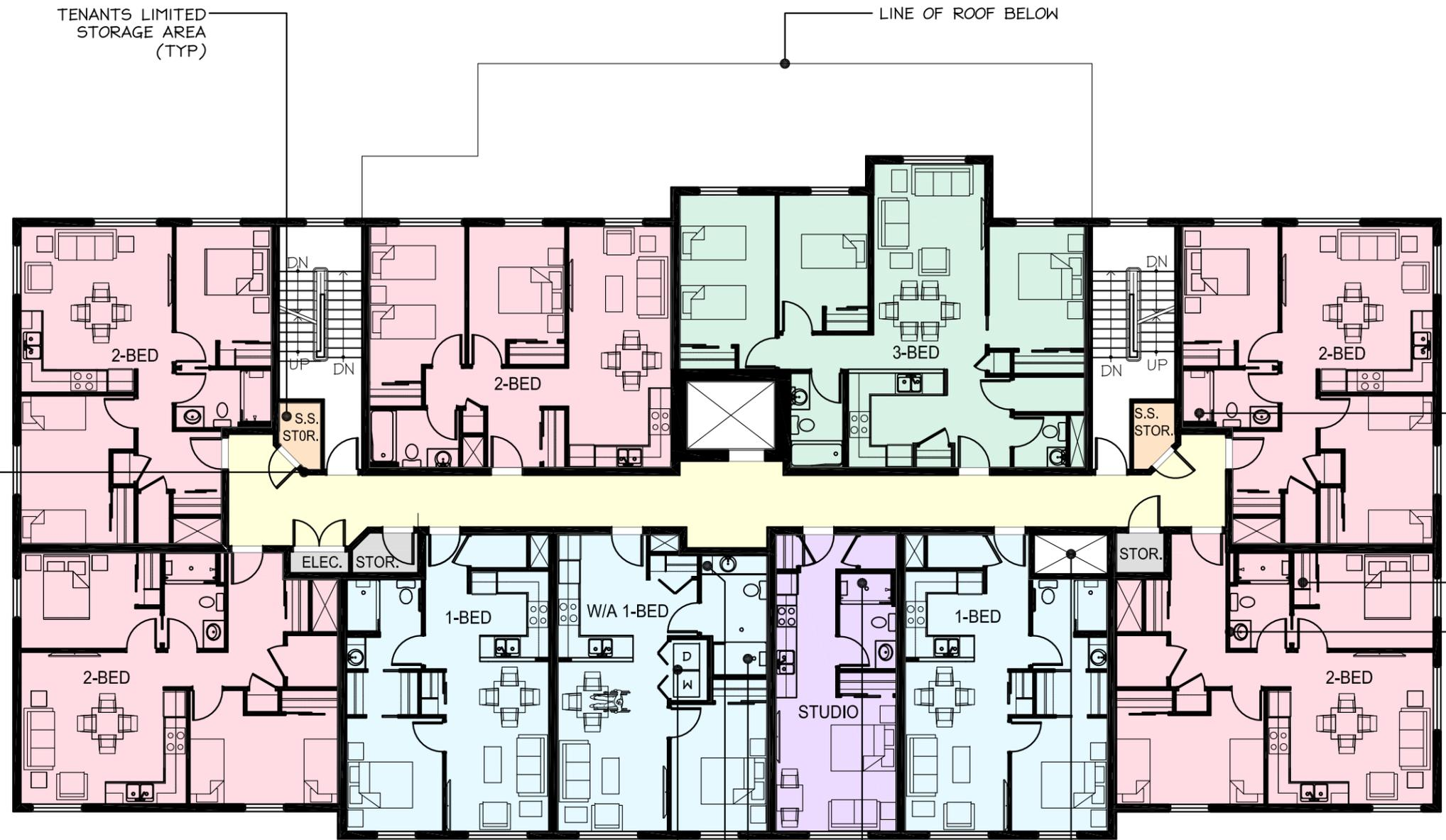
CHAMFERED WALLS CAN ASSIST IN BETTER VISIBILITY AT CORNERS TO IMPROVED SECURITY (TYP)
